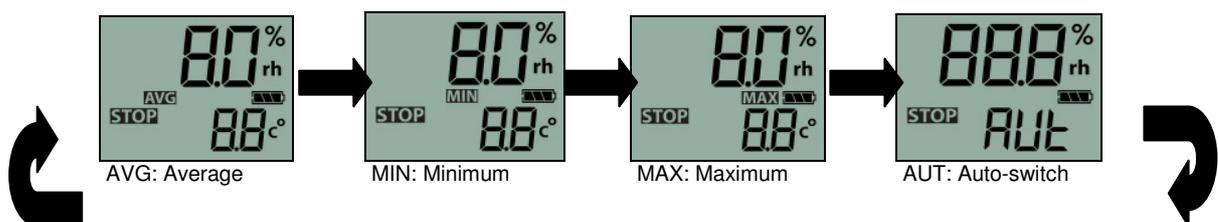
By using the AUTO-Mode(AUT) the display will switch automatically every two seconds.
